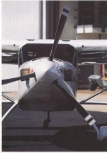
*The Comp Air 7 has a Walter turbine engine installed, which necessitated the very long cowling and the resulting pointed nose.*
