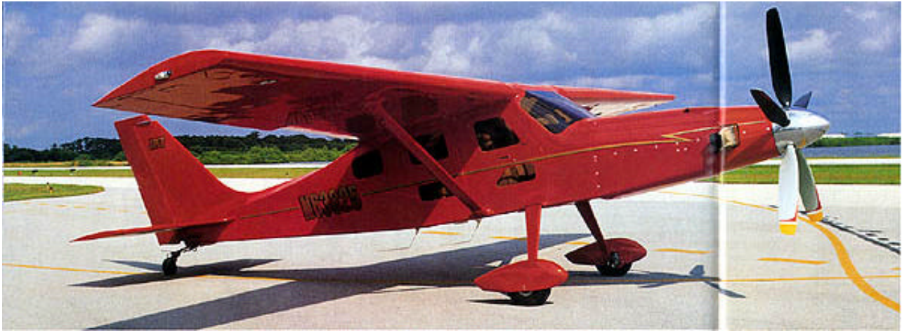
The long nose was necessary due to the length of the Walter engine and the need to place the lightweight power unit farther forward for aircraft balance.
