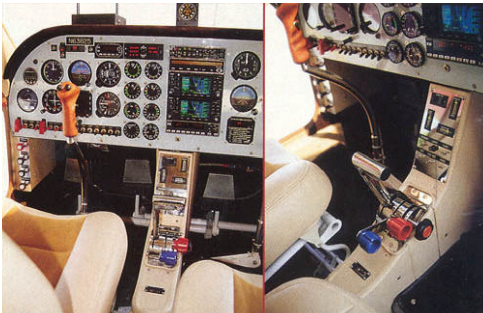
ABOVE LEFT: The instrument panel is large, allowing room for a wide range of avionics and instruments. The plane is flown with control sticks rather than control columns. ABOVE RIGHT: Turboprop engine controls are slightly different than those for reciprocating engines, but they're easy to learn.
