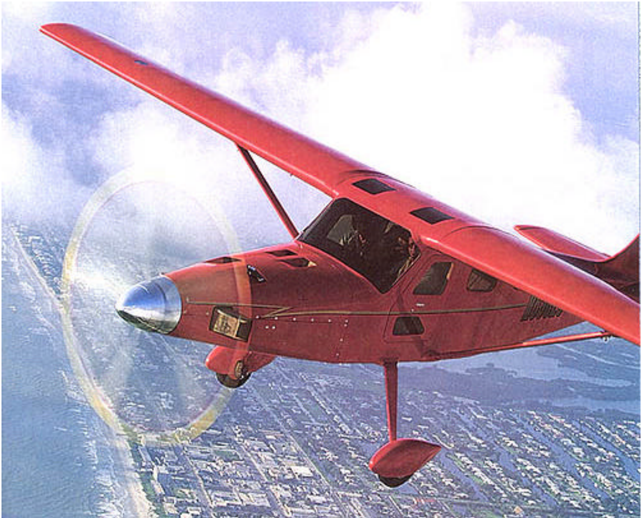
This Comp Air 7 Turbine has an Avia Hamilton five-blade prop swung by a 725-shp Walter 601 D water-injected engine. The aircraft has outstanding short-field performance and is easy to fly. It's available with tricycle gear.
