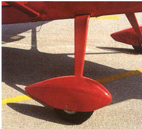
The rugged, forgiving landing gear on this Comp Air 7 Turbine was manufactured by Hammerhead Aviation in El Cajon, California.
