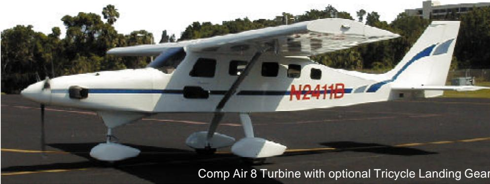
Comp Air 8 Turbine with optional Tricycle Landing Gear
