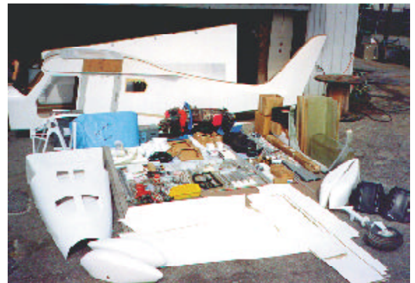
Comp Air 8 Turbine kit, including Walter M601D powerplant
